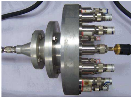
Figure 4. Photograph of the power divider under test.
