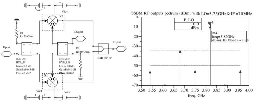
**Figure 1.** Microwave SSBM with more than 60 dB of LO suppression.
