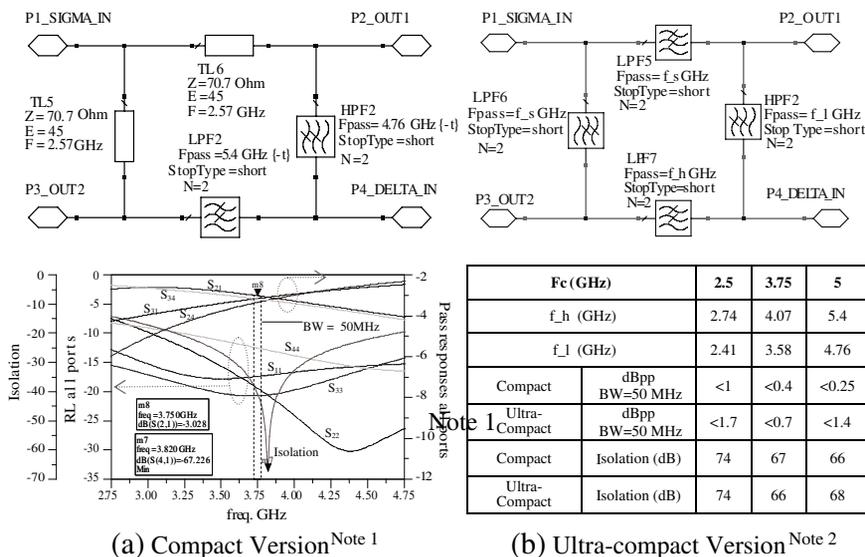
**Figure 2.** Ideal block diagrams of compact & ultra-compact hybrids, simulation plots of compact version and resuming table. (a) The length of the transmission lines on the schematic diagram was minimised to maintain the performance. The result was a 45° length line lower limit of operating frequency of hybrid (2.5 GHz). (b) The fixed corner frequency (f<sub>s</sub>) of the LPF-s between ports P1 & P2 and P1 & P3 of the schematic diagram was optimised on ADS to 4.5 GHz.
