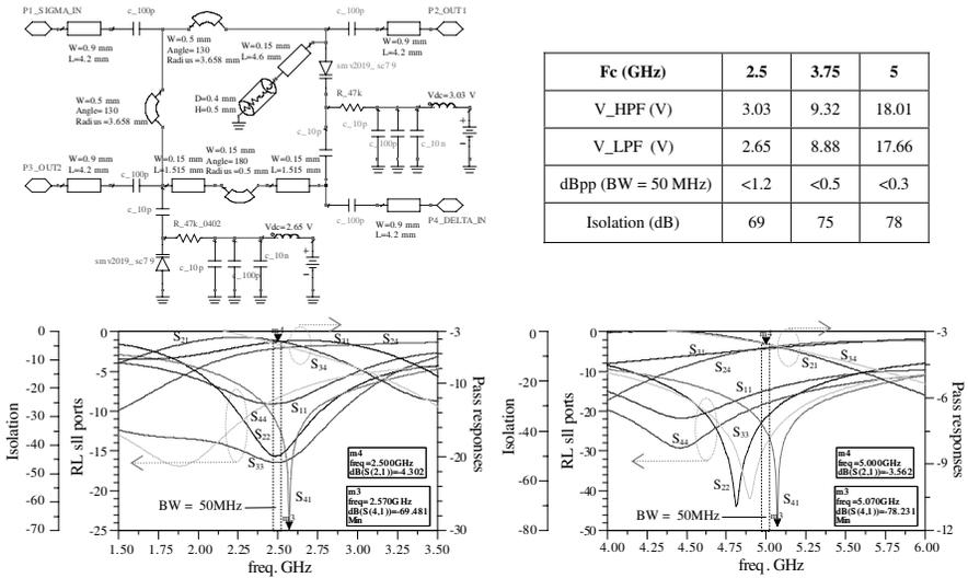
Figure 3. Schematic & quasi-realistic simulations of compact hybrid.
