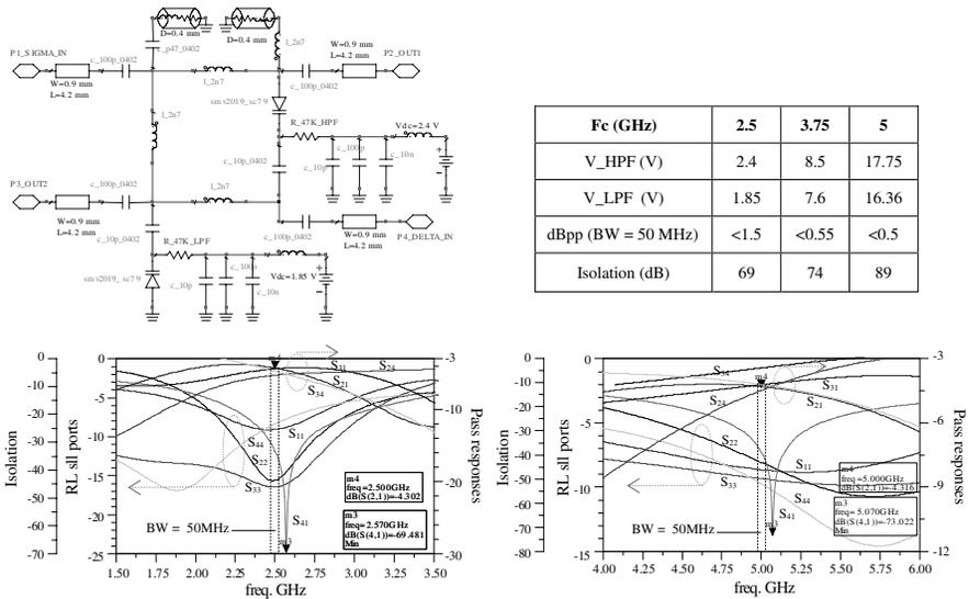
Figure 4. Schematic & quasi-realistic simulations of ultra-compact hybrid.
