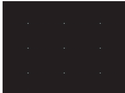
Figure 5. Imaging result of conventional DPCA SAR with full samples of raw data.
