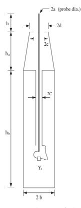
**Figure 5.** The cross sectional view of the structure (dimensions are:  $h = 5.35 \text{ cm}, h_b = 118.7 \text{ cm}, h_a = 14.6 \text{ cm}, a = 0.0787 \text{ cm}, b = 7.875 \text{ cm}, c = 0.2286 \text{ cm}, d = 4.25 \text{ cm}, e = 2.25 \text{ cm}.$ )
