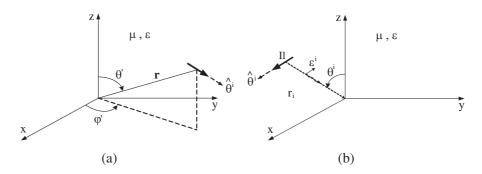
**Figure 4.** (a)  $\hat{\theta}^i$  directed dipole at the far zone. (b)  $\hat{\theta}^i$  directed dipole on xz plane at the far zone.
