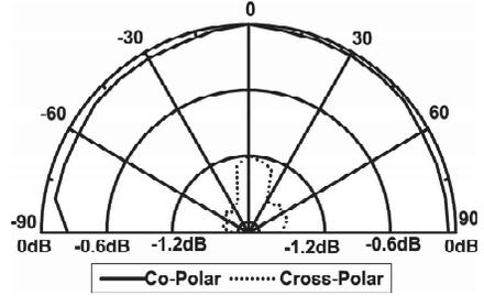
**Figure 18.** Radiation pattern of CTUAIURMSA when  $U_w = 0.2$  cm measured at 9.66 GHz.
