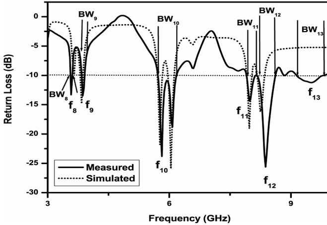
**Figure 6.** Variation of return loss versus frequency of CTUAIURMSA when  $U_w = 0.3$  cm.
