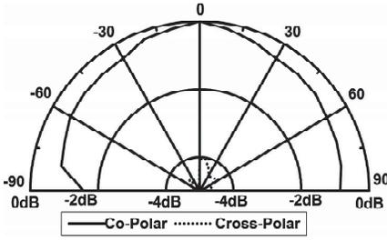
**Figure 27.** Radiation pattern of CTUAIURMSA when  $U_w = 0.1$  cm measured at 5.81 GHz.
