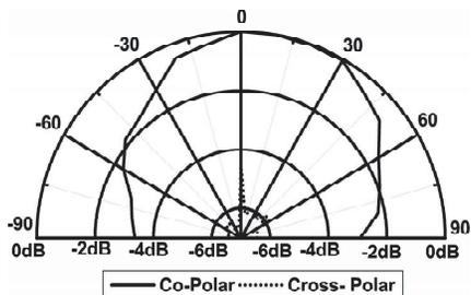
**Figure 26.** Radiation pattern of CTUAIURMSA when  $U_w = 0.1$  cm measured at 3.63 GHz.
