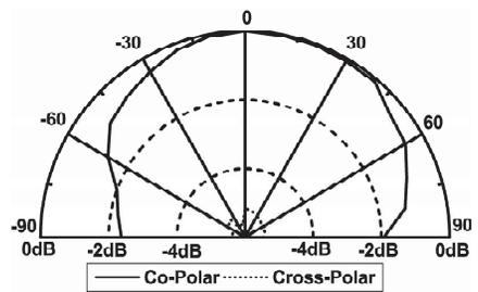
**Figure 20.** Radiation pattern of CTUAIURMSA when  $U_w = 0.3$  cm measured at 3.82 GHz.
