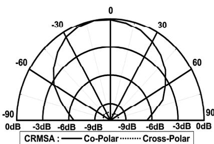
Figure 11. Radiation pattern of CRMSA measured at 3.39 GHz.
