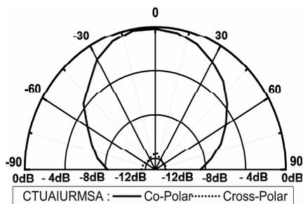
Figure 12. Radiation pattern of CTUAIURMSA when  $U_w = 0.2$  cm measured at 3.445 GHz.
