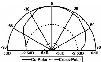
**Figure 21.** Radiation pattern of CTUAIURMSA when  $U_w = 0.3$  cm measured at 5.945 GHz.
