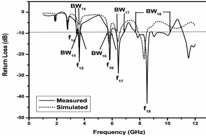
**Figure 7.** Variation of return loss versus frequency of CTUAIURMSA when  $U_w = 0.1$  cm.
