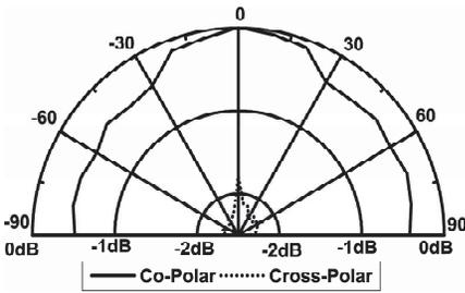
**Figure 17.** Radiation pattern of CTUAIURMSA when  $U_w = 0.2$  cm measured at 8.485 GHz.
