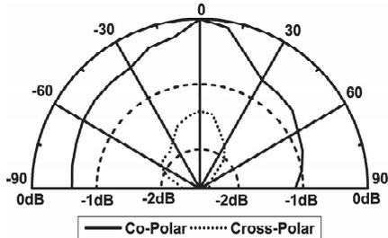
**Figure 22.** Radiation pattern of CTUAIURMSA when  $U_w = 0.3$  cm measured at 8.0 GHz.
