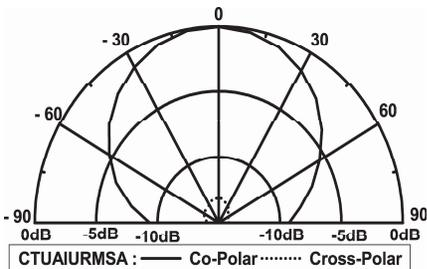
**Figure 19.** Radiation pattern of CTUAIURMSA when  $U_w = 0.3$  cm measured at 3.585 GHz.
