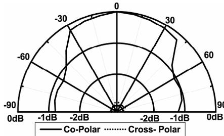
**Figure 29.** Radiation pattern of CTUAIURMSA when  $U_w = 0.1$  cm measured at 8.93 GHz.
