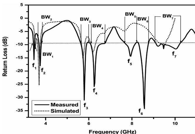
**Figure 5.** Variation of return loss versus frequency of CTUAIURMSA when  $U_w = 0.2$  cm.
