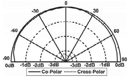
**Figure 28.** Radiation pattern of CTUAIURMSA when  $U_w = 0.1$  cm measured at 6.05 GHz.
