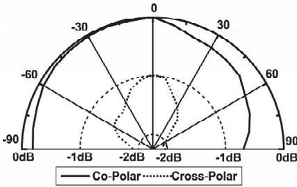
**Figure 15.** Radiation pattern of CTUAIURMSA when  $U_w = 0.2$  cm measured at 6.4 GHz.
