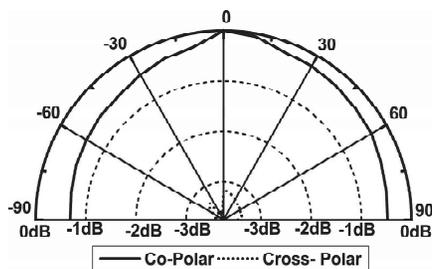
Figure 14. Radiation pattern of CTUAIURMSA when  $U_w = 0.2$  cm measured at 5.79 GHz.
