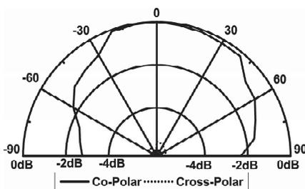
Figure 13. Radiation pattern of CTUAIURMSA when  $U_w = 0.2$  cm measured at 3.74 GHz.
