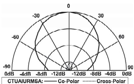
**Figure 25.** Radiation pattern of CTUAIURMSA when  $U_w = 0.1$  cm measured at 3.45 GHz.
