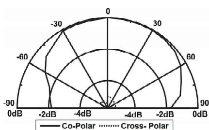
**Figure 24.** Radiation pattern of CTUAIURMSA when  $U_w = 0.3$  cm measured at 9.49 GHz.
