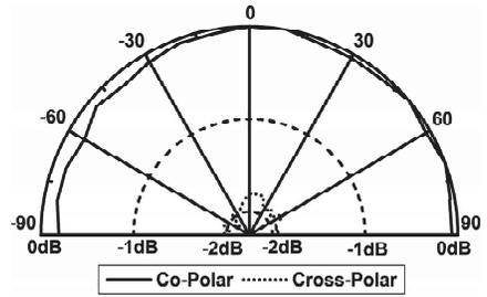
**Figure 16.** Radiation pattern of CTUAIURMSA when  $U_w = 0.2$  cm measured at 7.925 GHz.
