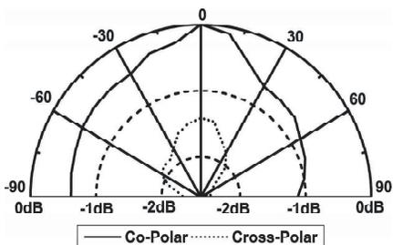
**Figure 23.** Radiation pattern of CTUAIURMSA when  $U_w = 0.3$  cm measured at 8.41 GHz.
