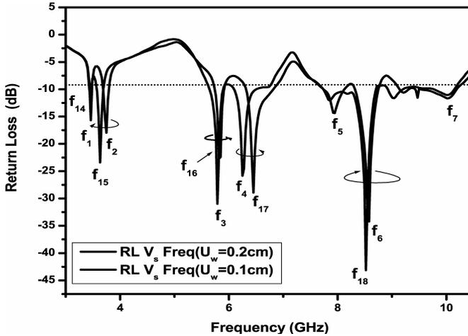
**Figure 9.** Comparison of experimental return loss versus frequency of CTUAIURMSA when  $U_w = 0.2$  and  $0.1$  cm.
