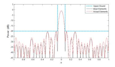
Figure 11. Pencil beam radiated by the isophoric phase-only reconfigurable array: (black curve)  $\sin \theta$  element pattern embedded; (red curve) realistic waveguide element pattern embedded.
