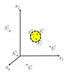
**Figure 3.** Representation, in the space of array locations, of: (green point) the unique solution of a pencil beam synthesis problem; (blue and red points) three equivalent solutions for two different shaped beams. The yellow set, achieved by minimizing (5), identifies the solutions most suitable for a 'common-locations' reconfiguration.
