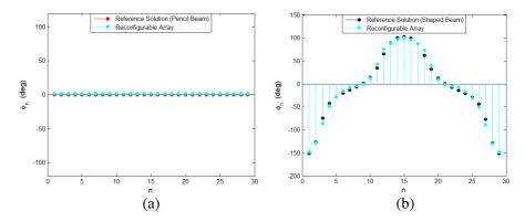
**Figure 10.** Isophoric array's excitation phases corresponding to: [(a), red lines] reference pencil beam; [(b), black lines] reference isoflux pattern; [(a), (b), cyan blue lines] phase-only reconfigurable patterns.
