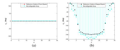
**Figure 6.** Isophoric array's excitation phases corresponding to: [(a), red lines] reference pencil beam; [(b), black lines] reference flat-top beam; [(a), (b), cyan blue lines] phase-only reconfigurable patterns.
