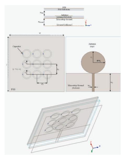
Figure 3. The proposed antenna and varactor tuned array.
