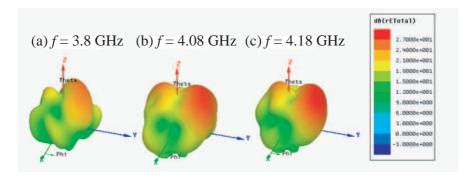
**Figure 5.** Computed radiation patterns (in dB) of the complete filtenna at different frequencies (corresponding to three reverse bias voltages). (a)  $f = 3.8 \,\text{GHz}$ . (b)  $f = 4.08 \,\text{GHz}$ . (c)  $f = 4.18 \,\text{GHz}$ .
