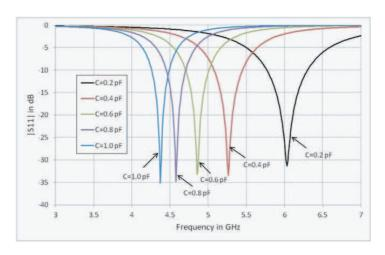
Figure 2. Simulated reflection coefficient of FSS with various capacitance values.
