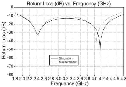
**Figure 14.** Simulated and measured return loss,  $f_c = 3.3$  GHz.
