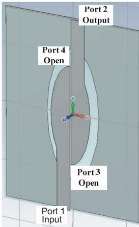
**Figure 2.** The proposed phase shifter is modelled as a four-port device, with two of the ports open circuited.
