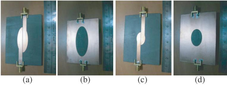
**Figure 9.** Photographs of the fabricated phase shifters. (a) Top layer,  $f_c = 1.65$  GHz. (b) Bottom layer,  $f_c = 1.65$  GHz. (c) Top layer,  $f_c = 3.3$  GHz and (d) Bottom layer,  $f_c = 3.3$  GHz.
