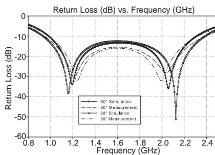
**Figure 11.** Simulated and measured return loss,  $f_c = 1.65$  GHz.
