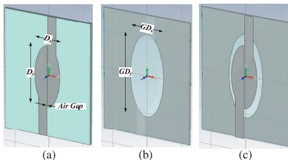
**Figure 1.** Configuration of the proposed phase shifter. (a) Top layer. (b) Bottom layer and (c) complete structure.
