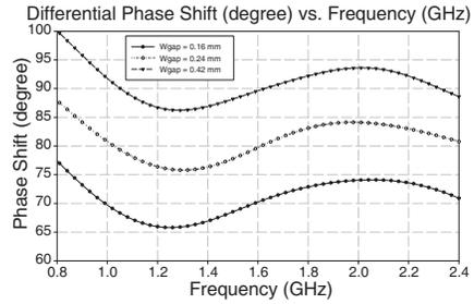
**Figure 3.** Simulated differential phase shift for varying gap width.
