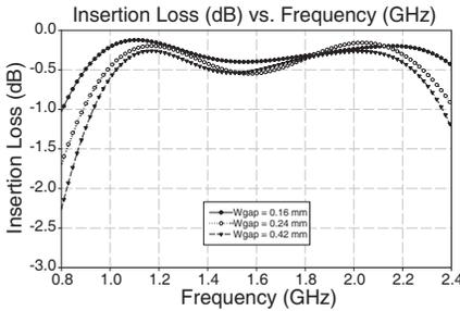
**Figure 4.** Simulated insertion loss for varying gap width.
