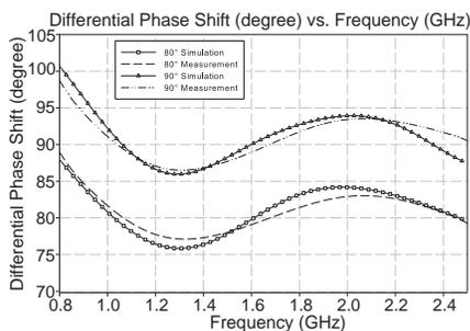
**Figure 10.** Simulated and measured differential phase shift,  $f_c = 1.65$  GHz.
