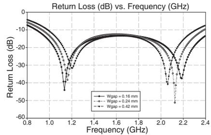
**Figure 5.** Simulated return loss for varying gap width.
