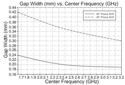
**Figure 7.** Gap width varies with center frequency for a certain amount of phase shift.
