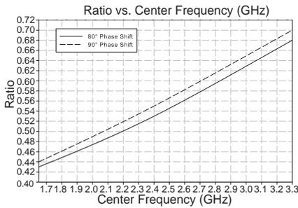
**Figure 6.** Ratio varies with center frequency for a certain amount of phase shift.
