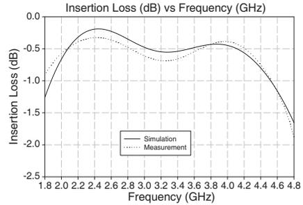
**Figure 15.** Simulated and measured insertion loss,  $f_c = 3.3$  GHz.
