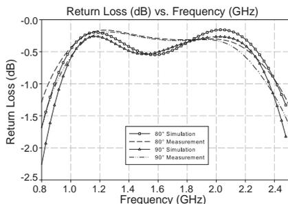
**Figure 12.** Simulated and measured insertion loss,  $f_c = 1.65$  GHz.
