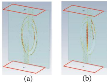
**Figure 8.** Surface current distribution (a)  $f = 0.95$  GHz and (b)  $f = 2.35$  GHz.
