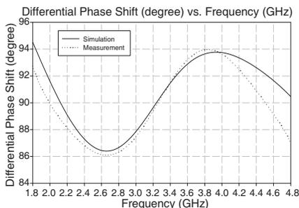
**Figure 13.** Simulated and measured differential phase shift,  $f_c = 3.3$  GHz.
