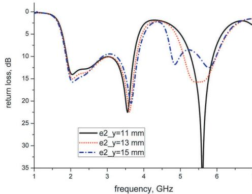
**Figure 6.** Return losses of the proposed antenna with various lengths of the inner oval-slot semi-minor axis  $e2_y$ ; other antenna parameters are given in Figure 2.
