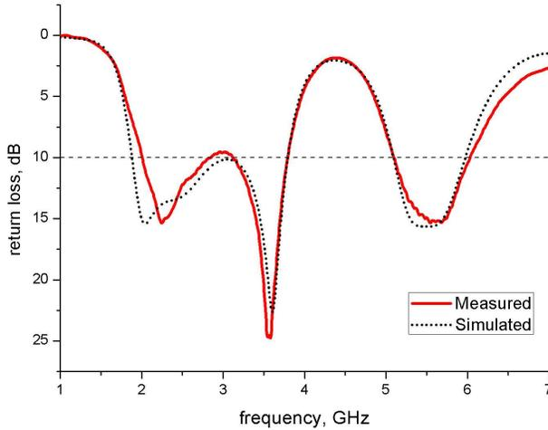
**Figure 2.** Measured and simulated return losses of the proposed antenna ( $e1_x = 17$  mm,  $e1_y = 20$  mm,  $e2_x = 16.5$  mm,  $e2_y = 13$  mm,  $e3_x = 11.5$  mm,  $e3_y = 15.5$  mm).
