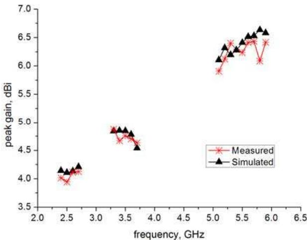
**Figure 8.** Peak gains of the proposed antenna for frequencies across 2.5, 3.5 and 5.5 GHz operating bands.
