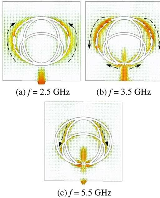
**Figure 3.** Simulated surface current distributions of the proposed antenna operating at 2.5, 3.5 and 5.5 GHz.
