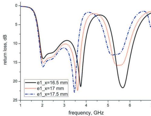
**Figure 4.** Return losses of the proposed antenna with various lengths of the outer oval-slot semi-minor axis  $e1_x$ ; other antenna parameters are given in Figure 2.
