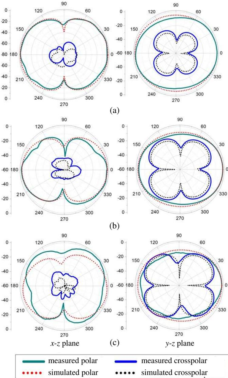
**Figure 7.** Radiation patterns of the proposed antenna. (a) 2.5 GHz. (b) 3.5 GHz. (c) 5.5 GHz.
