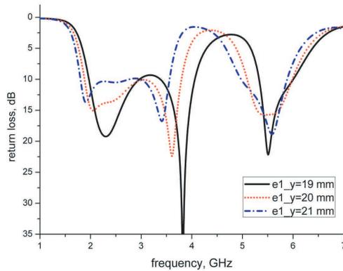
**Figure 5.** Return losses of the proposed antenna with various lengths of the outer oval-slot semi-major axis  $e1_y$ ; other antenna parameters are given in Figure 2.
