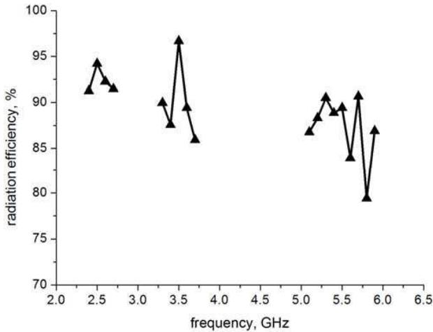
**Figure 9.** Simulated radiation efficiency for frequencies across 2.5, 3.5 and 5.5 GHz operating bands.
