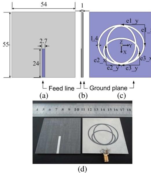
**Figure 1.** Configuration of the proposed crossed oval-ring slot triple-band antenna (units: mm). (a) Top view. (b) Side view. (c) Bottom view. (d) Fabricated antenna.
