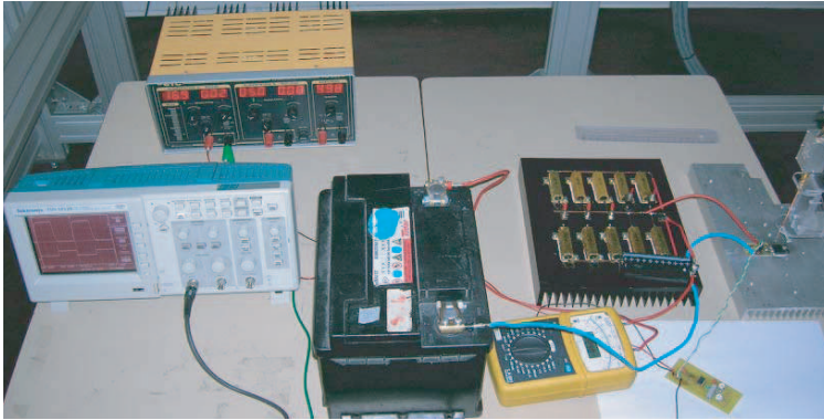
Figure 1. Experimental setup considered for the test of MOSFET.
