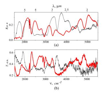
Figure 4. FTIR (a) Reflection and (b) Transmission spectra of the FP resonator with LC filler for E (thick line) and H (thin line) polarizations in the absence of an applied electric field. The resonator parameters are: width of Si walls,  $d_{Si} = 1 \,\mu\text{m}$ , cavity width,  $d_{cav} = 4 \,\mu\text{m}$ .
