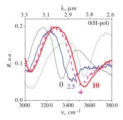
Figure 6. Smooth tuning of the position of the resonance peak from  $3330 \text{ cm}^{-1}$  to  $3550 \text{ cm}^{-1}$  for *E*- and *H*-polarization (dotted line). The applied voltage is shown in volts beside each curve.
