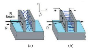
**Figure 1.** Schematic diagram of the Fabry-Pérot resonator, consisting of two Si walls separated by a gap infiltrated with liquid crystal molecules with (a) horizontal planar and (b) homeotropic alignment.
