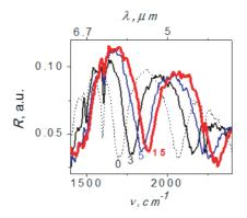
Figure 8. Smooth tuning of the resonance peak from 1700 to  $1880 \,\mathrm{cm}^{-1}$  in the experimental reflection spectra of the FP resonator (from Fig. 5) with a maximal relative shift of  $\Delta\lambda/\lambda = 10\%$ .
