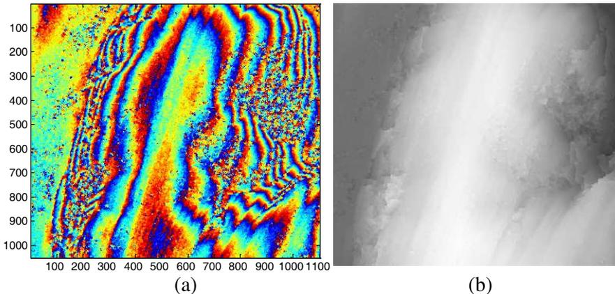
**Figure 4.** Interferogram and final unwrapped result. (a) Interferogram with flat-earth removed. (b) The unwrapped result using Flynn's minimum discontinuity algorithm.
