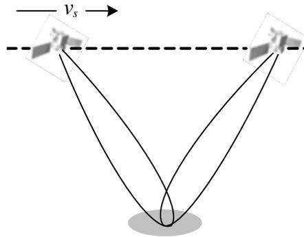
**Figure 1.** The geometry of spotlight SAR.
