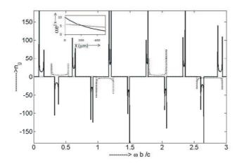
Figure 7. The variation of the effective group index  $n_g$  with respect to normalized frequency for P = 1,  $b = 500 \,\mu\text{m}$ , d = 1 with  $\alpha = 10$ ,  $\varepsilon_b = 2.04$  and  $\alpha = 6$ ,  $\varepsilon_b = 4.13$ .
