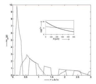
**Figure 5.** The variation of the effective phase index  $n_{eff}(p)$  with respect to normalized frequency for P = 1,  $b = 500 \,\mu\text{m}$ , d = 1 with  $\alpha = 10$ ,  $\varepsilon_b = 2.04$  and  $\alpha = 6$ ,  $\varepsilon_b = 4.13$ .
