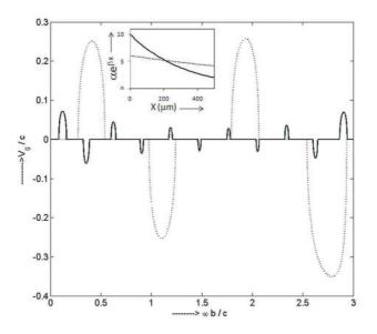
Figure 6. The variation of normalized group velocity with respect to normalized frequency for P = 1,  $b = 500 \,\mu\text{m}$ , d = 1 with  $\alpha = 10$ ,  $\varepsilon_b = 2.04$  and  $\alpha = 6$ ,  $\varepsilon_b = 4.13$ .
