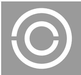
Figure 1. Schematic representation of CSRR.
