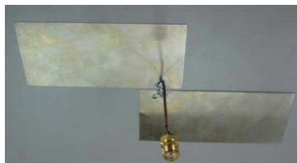
Figure 2. Photography of a coplanar-strip dipole antenna for CP operation.
