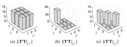
Figure 4. Absolute value of the correlation between transmit antenna elements shown in Figure 3.
