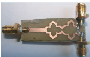
Figure 4. Photograph of 1.8 GHz power divider.
