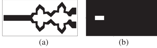
Figure 1. Layout of the proposed miniaturized Wilkinson power divider. (a) Top view. (b) Bottom view.
