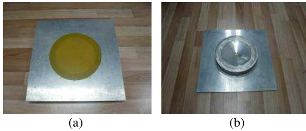
Figure 5. Photographs of the fabricated antenna with FRP and mounting plate. (a) Front view. (b) Back view.
