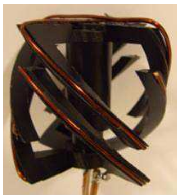
Figure 7. Photo of split QHA rotated ( 30^\circ around z -axis) and translated (24 mm along -z -axis) along with feed mechanism.
