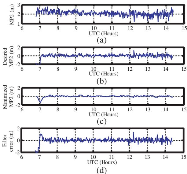
**Figure 4.** Multipath mitigation using LMS adaptive filter on  $L_2$  of SV17 (14 Aug. 2010). (a) Multipath error (MP2). (b) Desired MP2. (c) Minimized MP2. (d) Filter convergence error.
