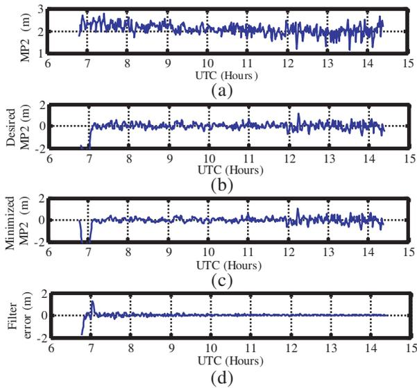
**Figure 6.** Multipath mitigation using RLS adaptive filter on  $L_2$  of SV17 (14 Aug. 2010). (a) Multipath error (MP2). (b) Desired MP2. (c) Minimized MP2. (d) Filter convergence error.
