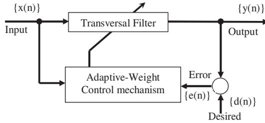
**Figure 2.** Typical block diagram of an adaptive transversal filter.
