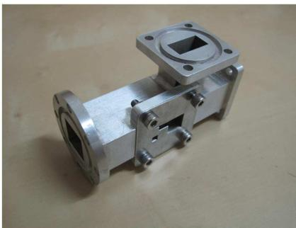
**Figure 5.** Photo of the fabricated OMT with an irregularly shaped diaphragm.
