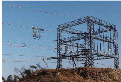
Figure 6. Field test of inspection robot with MFL sensor.
