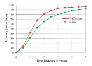
Figure 10. Accuracy comparison of two indoor positioning systems.
