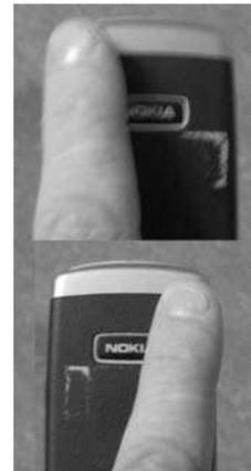
**Figure 3.** Capacitance output response measured in user's hand, index finger in turns located on right and left side of antenna. Measured finger locations on the backside of the phone are presented in detail.
