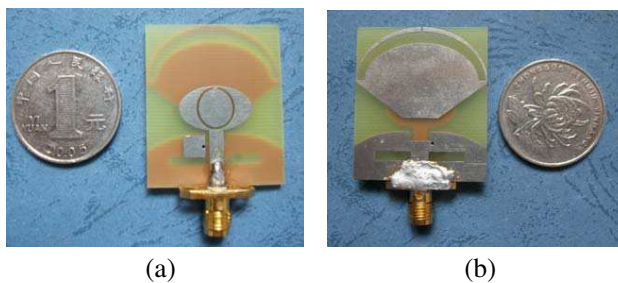
Figure 2. Photograph of the fabricated prototype. (a) Top view. (b) Bottom view.
