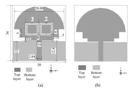
**Figure 1.** (a) Geometry of the proposed antenna. (b) Geometry of the reference antenna.
