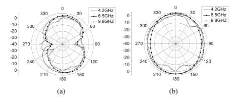
Figure 12. Measured radiation pattern of the proposed antenna. (a) E-plane (y-z plane). (b) H-plane (x-z plane).
