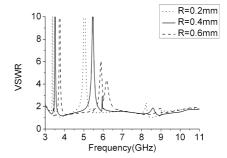
Figure 9. Simulated VSWR of the proposed antenna with various R.
