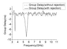
Figure 14. Measured group delay of the proposed antenna and the reference antenna.
