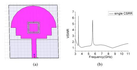
**Figure 3.** (a) Model of antenna with single CSRR. (b) Simulated VSWR of antenna with single CSRR.
