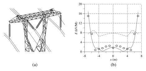
Figure 11. (a) Cross-arm of the 400 kV tower and (b) the electric field within this cross-arm. Continuous line — computations (influence of the tower truss is taken into account). Dash line — computations (influence of the tower truss is neglected). Circles — measurements on the real object.
