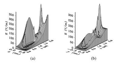
Figure 9. Computed electric field distribution around the model of human body that is located near the laboratory model of the transmission line. (a) For y = 0. (b) For x = 0.53 m.
