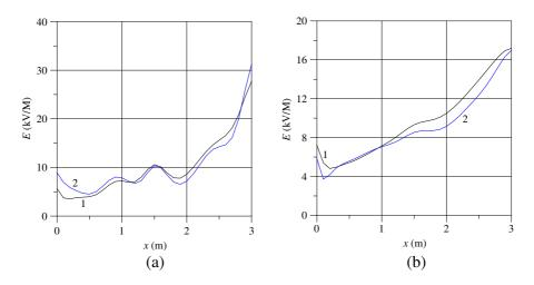
Figure 4. Electric field distribution near the detailed (1) and crude (2) model of the test object for y = 0, along x axis. (a) z = 0.25 m, (b) z = 0.5 m.
