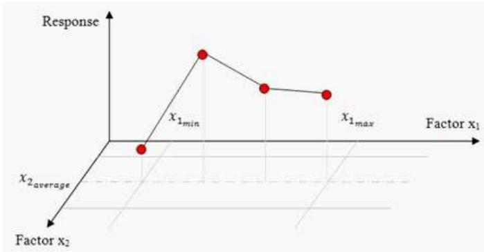
**Figure 1.** Traditional method of experiments.
