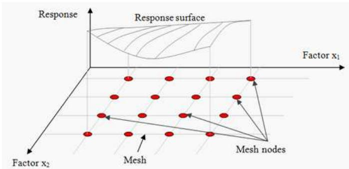
**Figure 2.** One experience at each node of the mesh.
