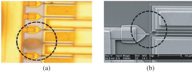
Figure 6. ESD induced failure (at 4 kV HBM ESD impulse). (a) Metallization burn-out, (b) line open.
