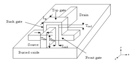
Figure 1. Schematic diagram of FinFET.
