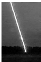
Figure 5. The video frame for the return stroke lightning channel during the triggered lightning experiment [18].
