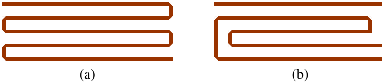
Figure 1. Two typical routing schemes for the delay line. (a) Serpentine routing scheme. (b) Flat spiral routing scheme.
