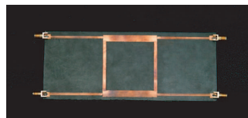
Figure 13. The top view of the fabricated coupler using ACNF.
