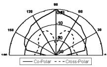
**Figure 7.** Radiation pattern of MPDRA at 7.07 GHz.
