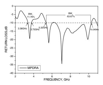
**Figure 3.** Plot of return loss (RL) versus frequency (GHz) response of MPDRA ( $h_{dr} = 6 \text{ mm}$ ).
