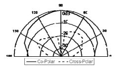
Figure 4. Radiation pattern of RDRA at 5.43 GHz.
