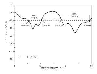
**Figure 2.** Plot of return loss (RL) versus frequency (GHz) response of RDRA ( $h_{dr} = 6 \text{ mm}$ ).
