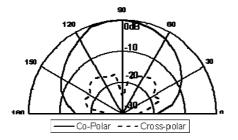
Figure 6. Radiation pattern of MPDRA at 3.57 GHz.
