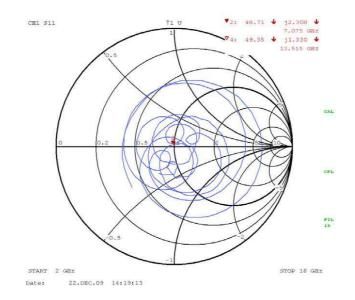
Figure 8. Measured input impedance characteristics on Smith chart.
