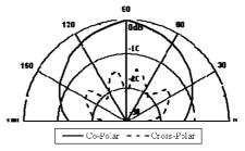
Figure 5. Radiation pattern of RDRA at 8.72 GHz.
