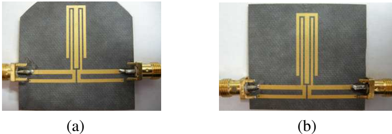
Figure 12. Photograph of the fabricated inductive S-L coupling dual-mode filters (a) L_2 = 21.5 mm; (b) L_2 = 23.1 mm.
