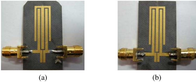
Figure 10. Photographs of the fabricated capacitive S-L coupling dual-mode filters, (a) L_2 = 21.15 mm; (b) L_2 = 22.04 mm.
