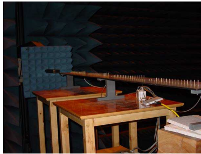
Figure 16. A S -band four elements end-fire array was under test.
