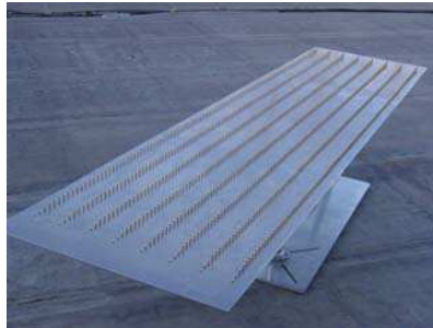
Figure 8. Eight elements end-fire array using the 120 monopoles plate end-fire antenna as the element.
