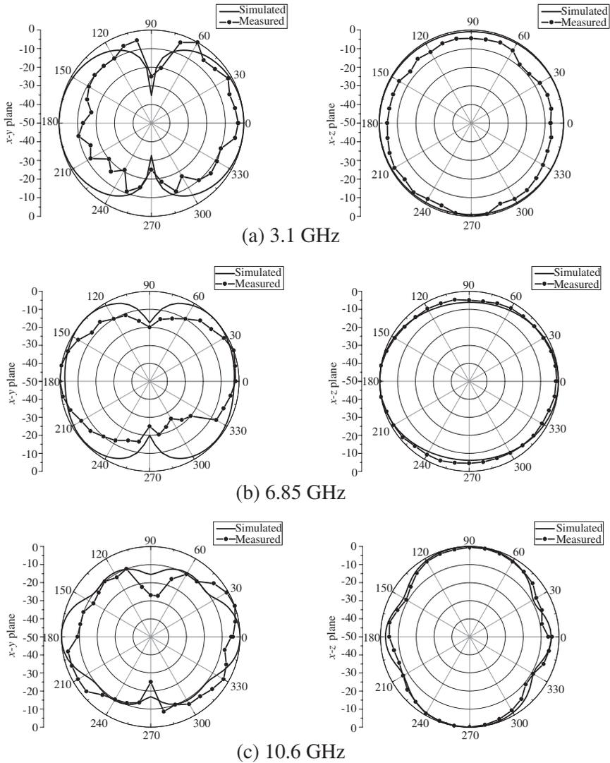
**Figure 5.** The simulated and measured results of antenna patterns.
