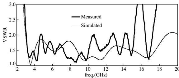
**Figure 4.** The simulated and measured results of antenna VSWR.
