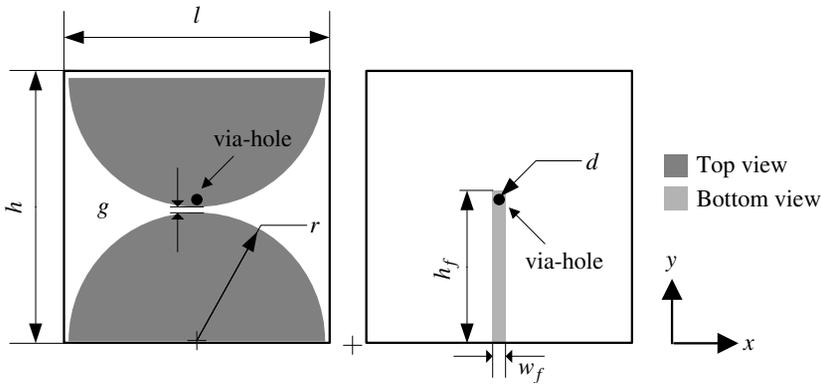
**Figure 1.** The sketch of the proposed antenna with associated geometrical parameters.  $h = 29.5$  mm,  $l = 29$  mm,  $g = 0.5$  mm,  $r = 14$  mm,  $d = 0.5$  mm,  $h_f = 16.5$  mm,  $w_f = 1.5$  mm.
