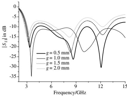
**Figure 2.** The simulated results of  $|S_{11}|$  with varying  $g$ .
