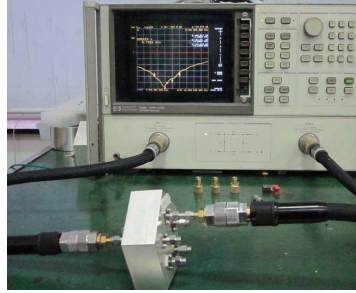
Figure 14. Five-way divider/combiner measurement setup.
