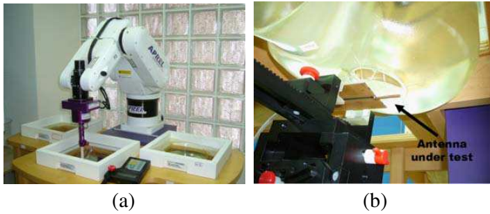
Figure 12. SAR test configuration: (a) Aprel ALSAS 10 SAR testing system, (b) the orientation of antenna and phantom model.
