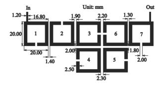
Figure 3. Physical dimensions of filter 1.
