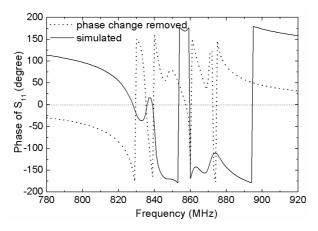
Figure 4. The  $S_{11}$  phase of filter 1 with and without removing the phase change.
