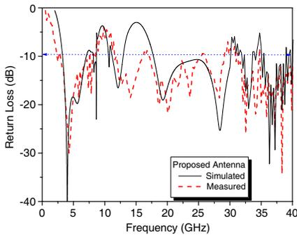
**Figure 2.** Simulated and measured reflection coefficient of the proposed antenna.
