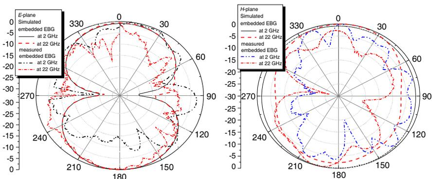
**Figure 8.** Comparison between measured and simulated *E*-plane and *H*-plane radiation patterns of embedded EBG with four arms spiral ground plane at two different frequencies.
