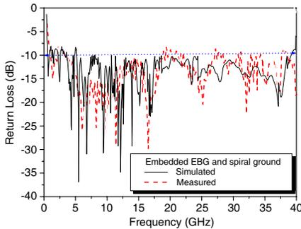
**Figure 6.** Comparison between simulated and measured reflection coefficient of embedded square EBG and four arms SDGS ground plane.
