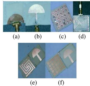
**Figure 7.** The fabricated proposed antenna (a) modified ground plane, (b) semi circular radiator, (c) embedded square EBG, (d) four arms SDGS, (e) embedded SDGS and (f) embedded square with four arms SDGS.
