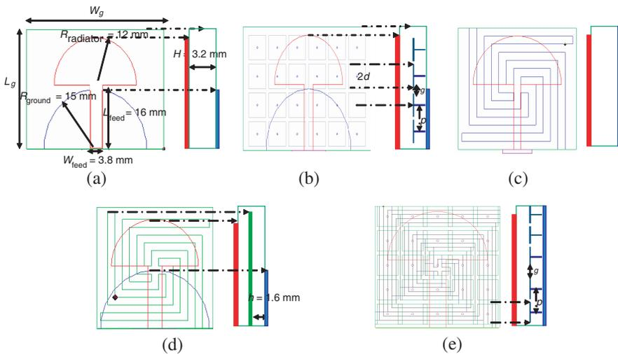
**Figure 1.** The prototype of the proposed antennas design. (a) Elevation and side view of proposed antenna. (b) Elevation and side view of antenna with EEBG. (c) Elevation and side view of antenna with SDGS. (d) Elevation and side view of antenna with embedded SDGS. (e) Elevation and side view of antenna with embedded EBG and SDGS ground.
