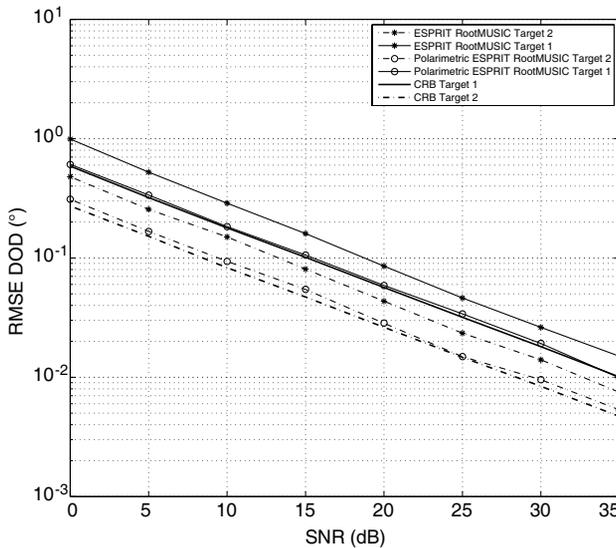
**Figure 3.** RMSE for DOD estimation versus SNR.
