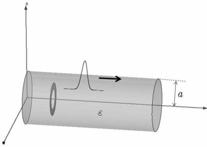
**Figure 1.** Circular dielectric waveguide.
