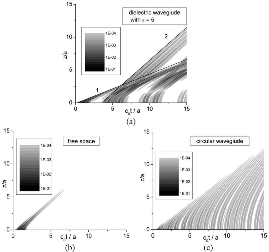
**Figure 3.** Amplitude distribution of longitudinal electric field component in  $z$ - $t$  coordinates at  $z$ -axis (a) for dielectric rod with  $\varepsilon = 5$ , (b) for free space, and (c) for closed hollow circular waveguide.
