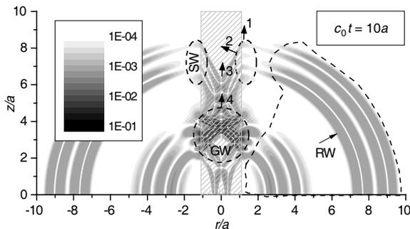
**Figure 5.** Distribution of longitudinal electric field component in  $r$ - $z$  coordinates at time instant  $c_0 t = 10a$  for dielectric rod with  $\epsilon = 5$ .
