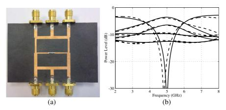
Figure 7. Power divider with 1:4:2:8 power ratio. (a) A photograph of the fabricated structure. (b) Simulation (ADS Momentum) and measurement results. Dashed lines are measured and solid lines are simulated power levels.
