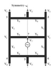
Figure 1. Seven ports power divider. The transmission lines joining adjacent ports are  $\lambda/4$  long at the center frequency.
