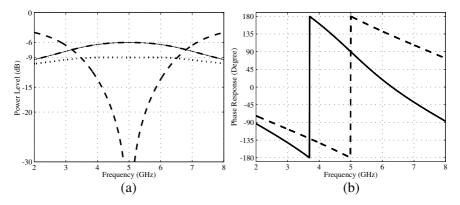
**Figure 3.** Simulation results for an ideal power divider with 1:2:1:2 power ratios in dB relative to input power. (a) Solid curve is the output power level at  $P_2$  and  $P_5 = -6$  dB. Dotted curve is the output power level at  $P_1$  and  $P_4 = -9$  dB. Dashed curve is the reflection coefficient  $|S_{77}|^2$ . (b) Solid line is the phase response of  $S_{27}$  and  $S_{57}$ , and dashed line is the phase response at ports  $S_{17}$ ,  $S_{37}$ ,  $S_{47}$ , and  $S_{67}$ .
