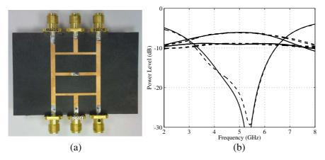
Figure 6. Power divider with 1:2:1:2 power ratio. (a) A photograph of the fabricated structure. (b) Simulation (ADS Momentum) and measurement results. Dashed lines are measured and solid lines are simulated power levels.
