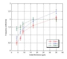
Figure 5. Frequency blueshift of the transfer functions of the filter sample 1, 2 and 3 of the batch A as a function of the metal sheet thickness.
