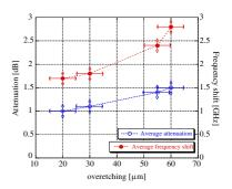
Figure 7. The average frequency shift and the attenuation of the filters 1, 2 and 3 of the batch B. While the attenuation is significantly affected by the size of the overetching, the effect on the frequency is small if compared to that due to the metal sheet thickness in the thickness range reported in Figure 5.
