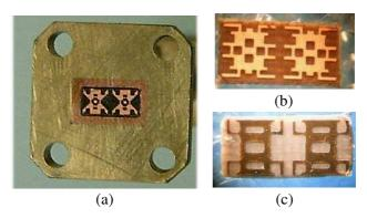
Figure 2. The composite material consists of two square cells with a side of 3.556 mm placed along the transverse direction of the Ka waveguide. (a) Picture of a sample accommodated in the waveguide. (b) Realized sample of the filter 2, and (c) filter 3.
