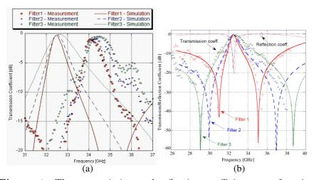
Figure 4. The transmission and reflection coefficient as a function of the frequency for three filter samples (1, 2 and 3) of the Batch A with  $t = 17 \,\mu\text{m}$ , compared with the simulations. (a) Comparison between the original experimental (dotted) and simulated (line) TF. (b) Agreement between the measured and the simulated transfer function shape after rigid frequency shift of the former.
