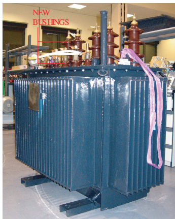
Figure 15. High voltage transformer used for the experimental tests.
