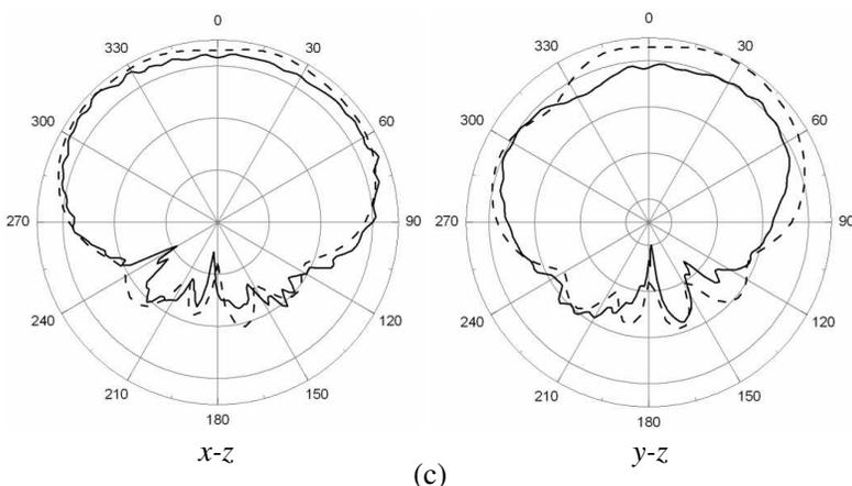
**Figure 6.** Radiation patterns for the proposed antenna (measured (—) and simulated (- -)). (a) 2.45 GHz, (b) 5.2 GHz, (c) 5.8 GHz.
