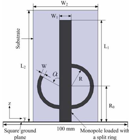
**Figure 1.** Geometry of proposed monopole antenna loaded with a split ring. All dimensions are:  $L_1 = 24.7$  mm,  $W_1 = 3$  mm,  $L_2 = 27.2$  mm,  $W_2 = 16.2$  mm,  $R = 4.7$  mm,  $W = 0.9$  mm,  $R_0 = 8.8$  mm,  $\alpha = 50$  deg.
