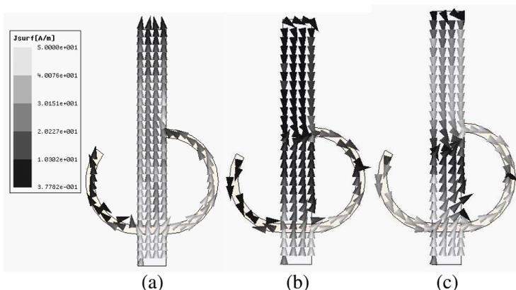
**Figure 5.** Simulated surface current distributions at different frequencies. (a) 2.45 GHz, (b) 5.2 GHz, (c) 5.8 GHz.
