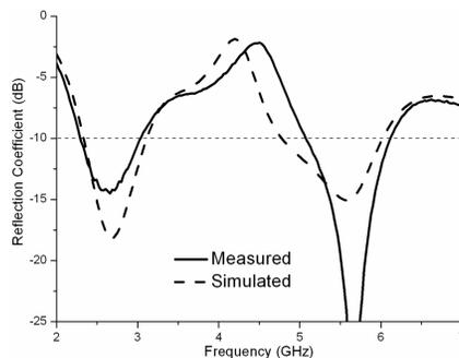
**Figure 4.** Measured and simulated reflection coefficient for the prototype antenna whose dimensions are shown in Fig. 1.
