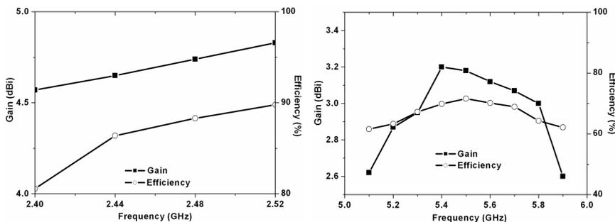
**Figure 7.** Measured peak gains and radiation efficiencies across the operating frequencies.
