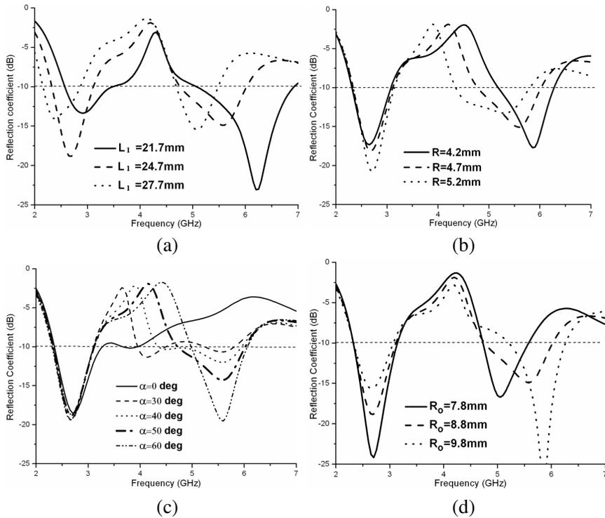
**Figure 2.** Parametric study of the variation of reflection coefficient with respect to (a) the monopole length  $L_1$ , (b) the split ring radius  $R$ , (c) the split angle  $\alpha$ , and (d) the split ring offset  $R_0$ .
