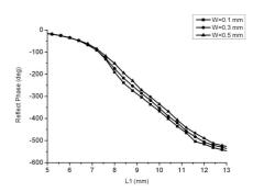
Figure 5. Phase responses of the proposed element for different W at the center frequency of 10 GHz  $(H_1 = 2 \text{ mm}, H_2 = 3 \text{ mm}, \text{ and } K = 0.66).$
