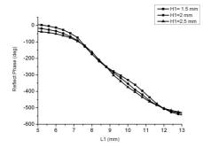
Figure 2. Phase responses of the proposed element for different  $H_1$  at the center frequency of 10 GHz  $(H_2 = 3 \text{ mm}, K = 0.66, \text{ and } W = 0.3 \text{ mm}).$
