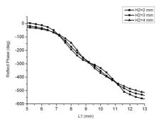
Figure 3. Phase responses of the proposed element for different  $H_2$  at the center frequency of 10 GHz  $(H_1 = 2 \text{ mm}, K = 0.66, \text{ and } W = 0.3 \text{ mm}).$
