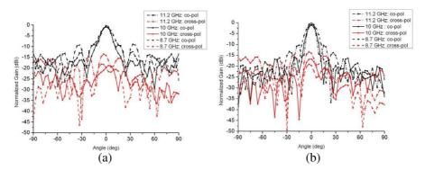
Figure 8. The measured radiation patterns at 8.7, 10, and 11.2 GHz for the designed 77-element linear reflectarray: (a) *E*-plane, (b) *H*-plane.
