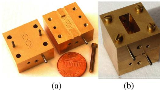
**Figure 5.** Photograph of the copper block with holes and waveguides for the channel-drop filter and scale. (a) The top and bottom halves of the block are shown separately. (b) The top and bottom halves of the block are connected together with screws.
