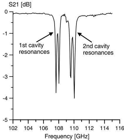
**Figure 12.** Measured transmission through the electroformed CDF with one cavity detuned by a copper rod inserted in the center. Four dips correspond to the filter resonating in each of the four partial eigenmodes of the two micro-cavities.
