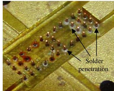
**Figure 8.** Photograph of the channel-drop filter with soldered rods. The filter is cut apart with electro-discharge machining. Solder penetration from the outside is clearly visible.
