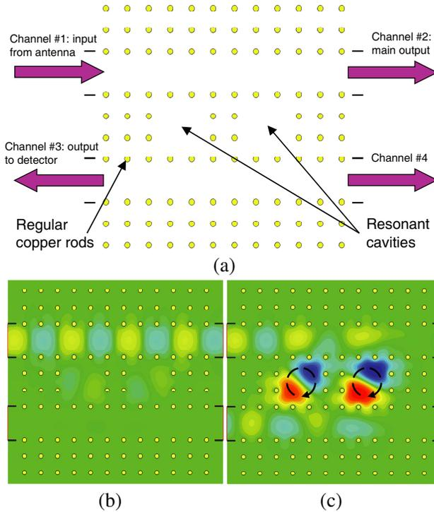
**Figure 1.** (a) Schematic of a channel-drop filter. (b) Electric field amplitude for the nonresonant frequency. Power transmits straight into channel #2 for nonresonant frequencies. (c) Electric field amplitude for the resonant frequency. The field pattern rotates in the direction of the arrows. At resonance the power transmits into channel #3 through the resonant cavities.
