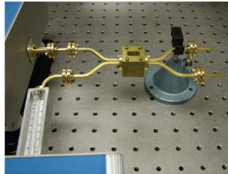
**Figure 6.** Photograph of the measurement set-up in the mm-wave laboratory.
