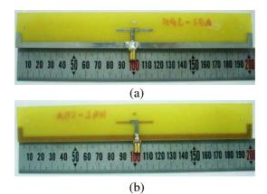
**Figure 6.** The prototype of the proposed antenna, (a) Front-view, (b) Back-view.
