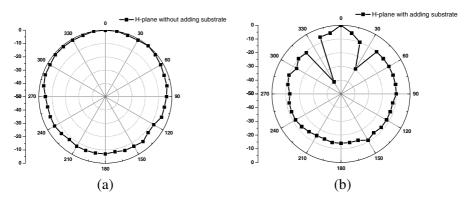
Figure 10. The measured results of radiation pattern in H-plane. (a) H-plane without adding substrate. (b) H-plane with adding substrate.
