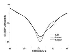
Figure 3. The simulated results of reflection coefficient with varying folded length.
